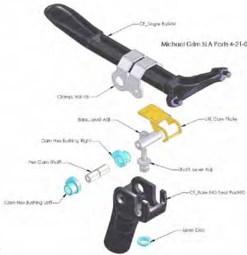
New "I-Beam" bike seat post concept.
